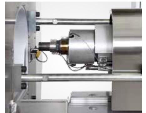
Optimized process control thanks to actively controlled nozzle needle valve
