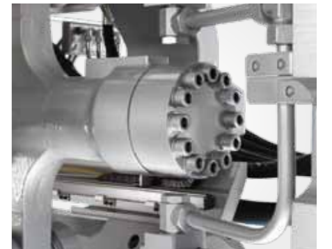
Reduced footprint thanks to inward-facing closing cylinder
