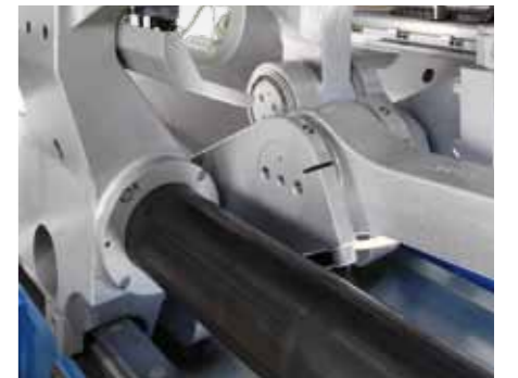
Transfer of force through centrally inclined 5-point toggle lever
