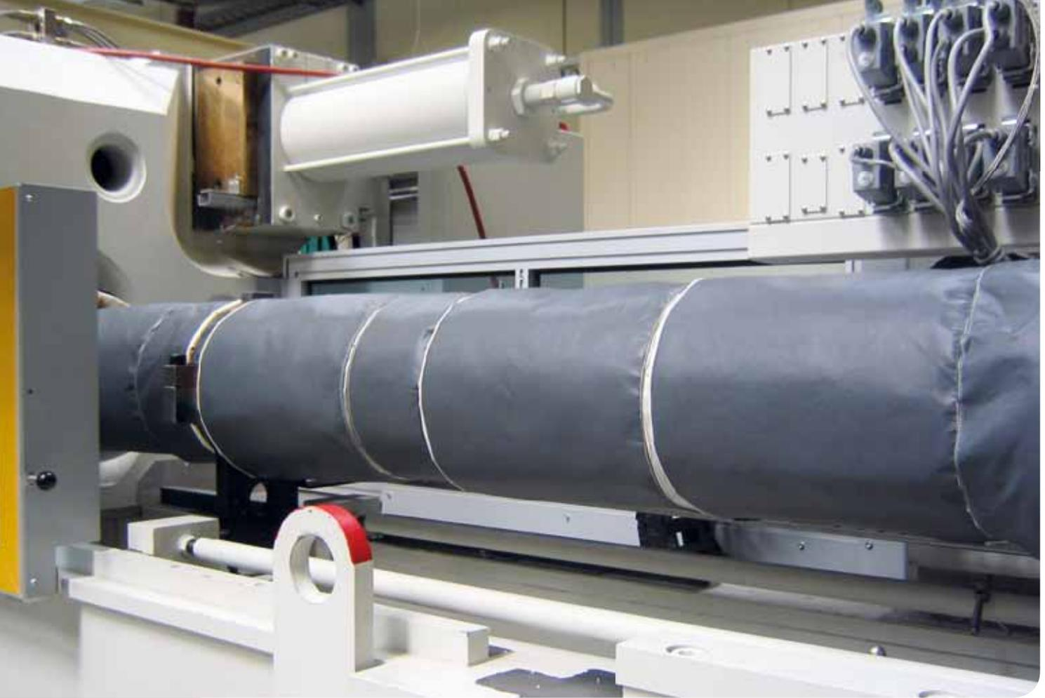
Fig. 9: Barrel insulation with KraussMaffei Ecopac barrel sleeves can reduce energy consumption for heating by 20 to 40%.
