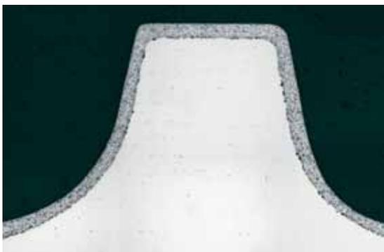
Fig. 18: Cross-section through part of a screw with thin hard-coating layer, coating thickness 0.3 mm
