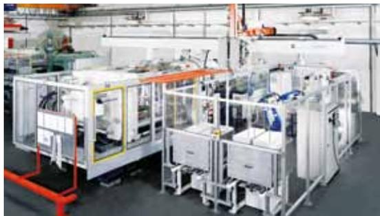
KM 650-5700 DF manufacturing cell for automotive pillar trim (Montaplast)
