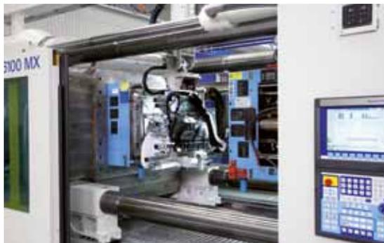
Big MX Series machine with DecoForm® module producing automotive door trim panels with sensitive décor materials
