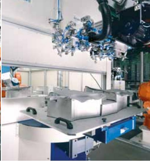
Automated transfer to laser trimming unit
