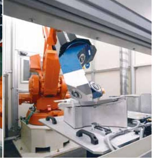
Laser edge trimming for pillar elements
