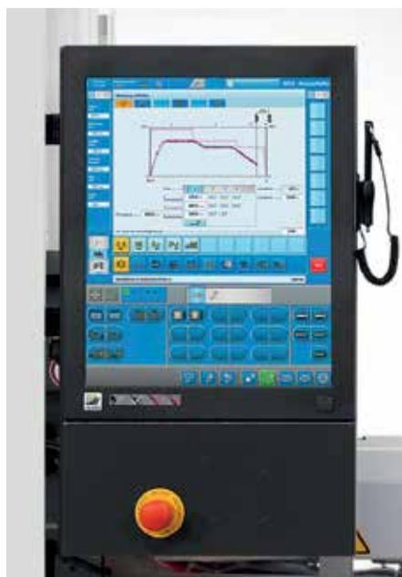
All process parameters can be set centrally from the MC6 control system using the special MuCell® controller
